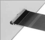
3 Rotate down the actuator until firmly closed. It is critical that the inserted FPC is not moved and remains fully inserted.
