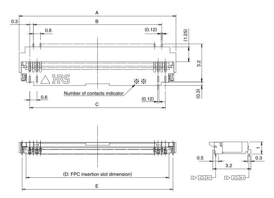
Notes 1 The coplanarity of each terminal lead within specified dimension is 0.1 mm Max.
