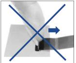
♦FPC Insertion(1) The FPC should be aligned parallel with the board surface and perpendicular with the connector (as shown), then completely inserted.
